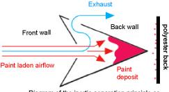
Diagram of the inertia separation principle as
